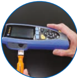
Replaceable RJ45 contacts
