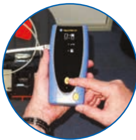
Autotest from remote unit for one person testing
