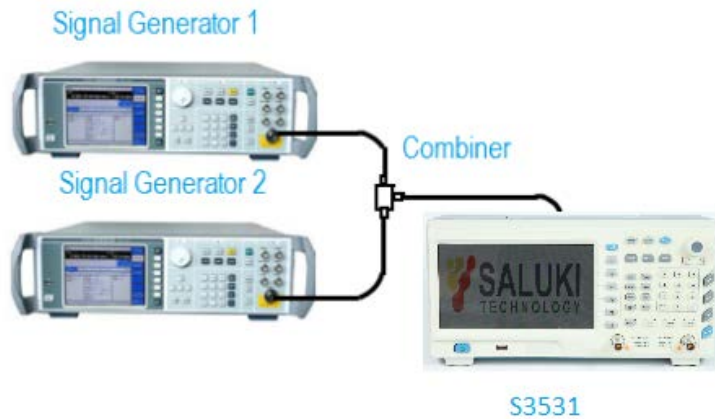
Fig 5-2: Equipment Connection for 2 signal capture
